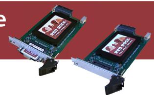
The 3U VPX SATA drive module provides storage using COTS 2.5" Hard Disk Drives (HDDs) or Solid State Drives (SSDs) with a range of capacity, speed, environmental, security and cost options.
